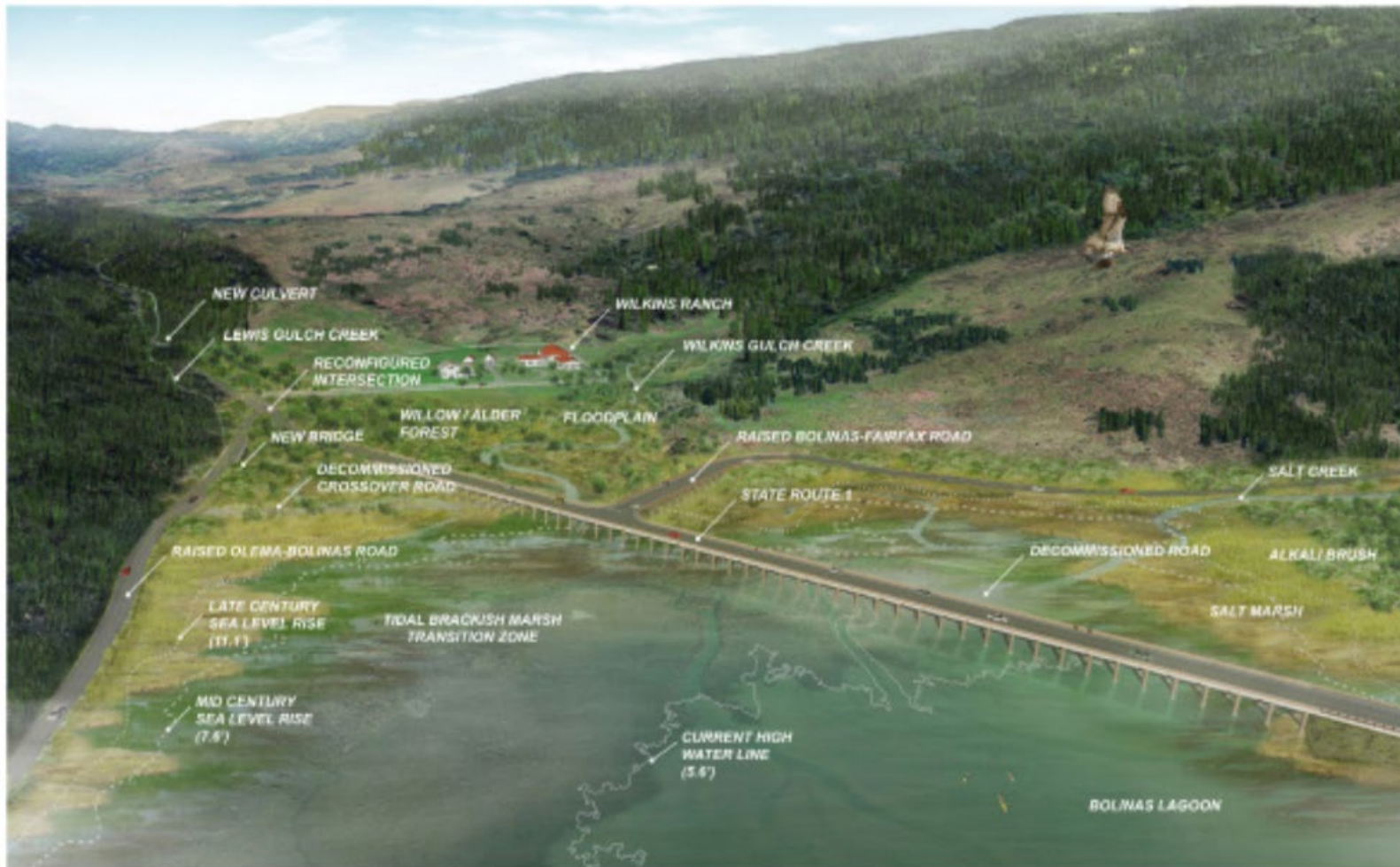
The Bolinas Lagoon North End Project includes a suite of changes to local roads, wetlands, and streams to reduce flooding and make them more resilient in the face of the additional 3–5 feet of sea level rise expected over the next century.
